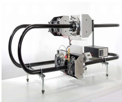
Figure 1.7: Schematic drawing of solar powered thermoacoustic cooler developed in the aster-thermoacoustics company
