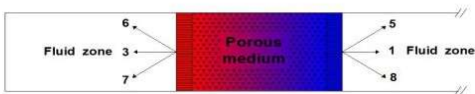
Figure 2.6: Illustrative drawing of basic lattices used for fluid-solid interface treatment
