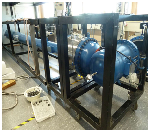
Figure 1.9: Thermo-acoustic heat pump developed by the TASTE project
