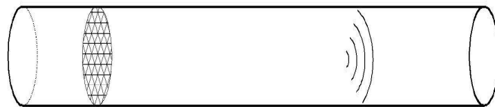
Figure 1.2: Structure of Rijke tube
